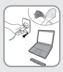
Disconnect all cables connected to the computer before cleaning it. If your notebook is external & removable battery type, remove the external battery.
